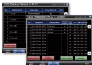
iQSS backup/restoration (PLC↔sensor) function
