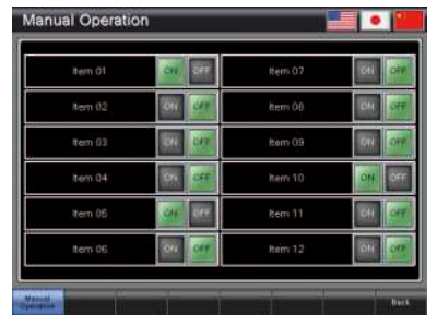
Manual operation (6 patterns) Executes ON/OFF operations of signals (bit devices)
