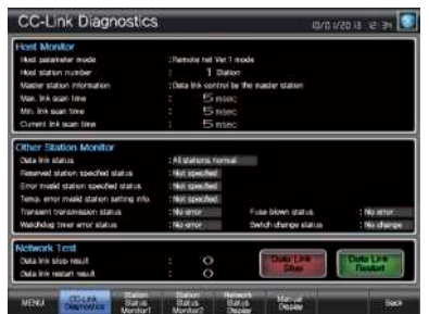
CC-Link network monitor Displays the CC-Link network status (host station, other stations, errors, etc.)
