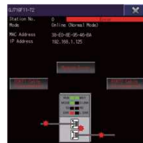
Communication status monitor window
