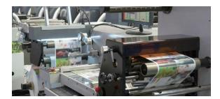
SSCNET III/H allows configuration of a multi-axis synchronous control system even for unwinders and rewinders with multiple axes. For machines with a machining axis, further high-level synchronous control system is possible by using cam control and advanced synchronous control.
